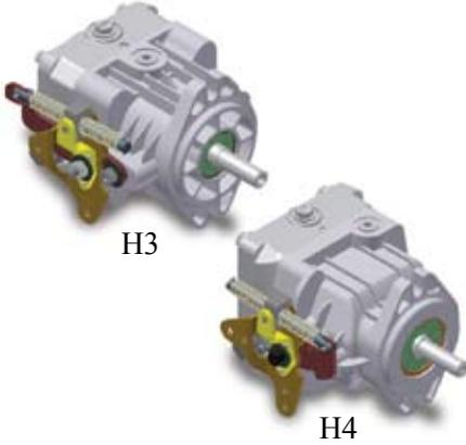
The H3 and H4 Series are manually controlled closed loop axial piston pumps. When paired with Parker's low speed, high torque orbit - type hydraulic motors, they create highly efficient hydrostatic transmissions. These cost effective transmissions are often used as drive systems for the propulsion of off - highway vehicles under 50 horsepower
