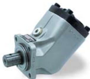
F1 fixed displacement piston pumps are widely used on truck applications with operating pressure up to 5000 PSI. These lightweight, efficient pumps were designed specifically for truck applications including cargo cranes, hook loaders, forest cranes and concrete mixers.
