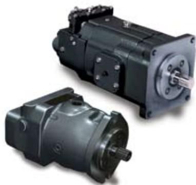
The Gold Cup Hydrostatic Transmission pumps are variable displacement piston pumps of an unparalleled rugged design. Rated to 5000 PSI continuous pressure and continuous duty, the Gold Cup design has the unique feature of an internal servo/replenish and the ability to utilize system over pressure to directly control the stroking chambers. This affords the fastest and most stable control strategy available.
