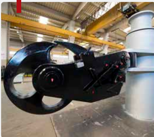
Towing hook foundation with integrated manoeuvring capstan
