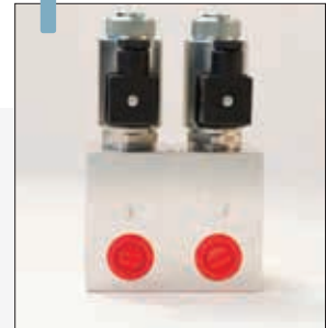
DKV-4E 24VDC electric activated valves are integrated on DKV-4. It is used in systems with a HPU. Electric activated valves are normally open. They are closed automatically when HPU valves are activated to prevent conflict between power operated system and manual helm pump which may cause oil loss in helm pump reservoir. DKV-5E is the version without DKV-4 and it is equipped with only electric activated valves. Material is marine grade aluminium.
