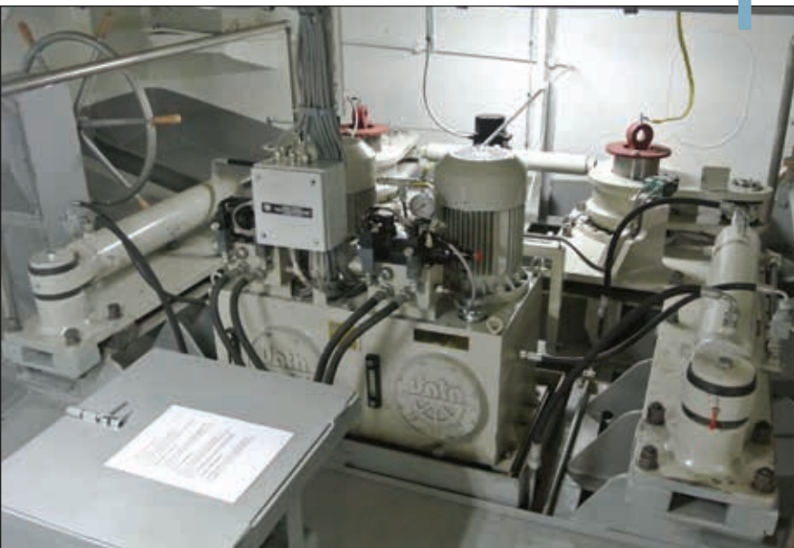
DDM 2x4000 custom design steering gear on a ferryboat
